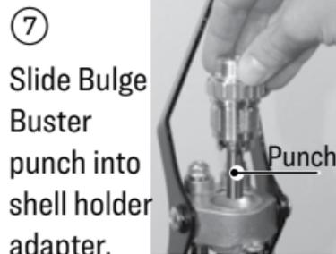
Assemble the Bulge Buster and Carbide Factory Crimp Die.
