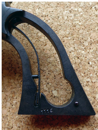
The mainspring is slotted into the frame
