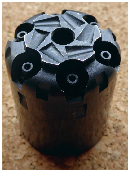
The rear of the cylinder, note the safety notches and angled nipples
